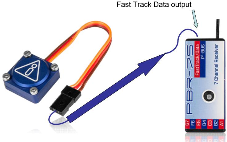
Power Box Systems doesn't offer receivers with integrated Gyros. They offer the "I Gyro Sat" which has to be connected to the "FastTrack/Data" output.
